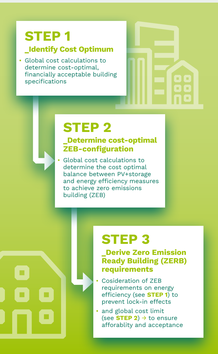
Figure 2-1 _Methodology to identify Zero Emission Building (ZEB) requirements adapted to MENA countries
