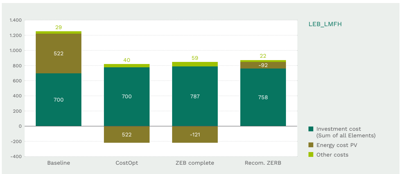
Figure 2-30 _Global cost comparison most relevant variants, including baseline and the recommended ZERB
